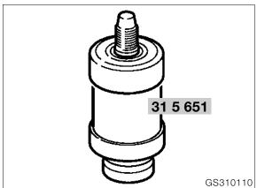
Press out the threaded pin using a mandred, BMW No. 31 5 651, as a support.
