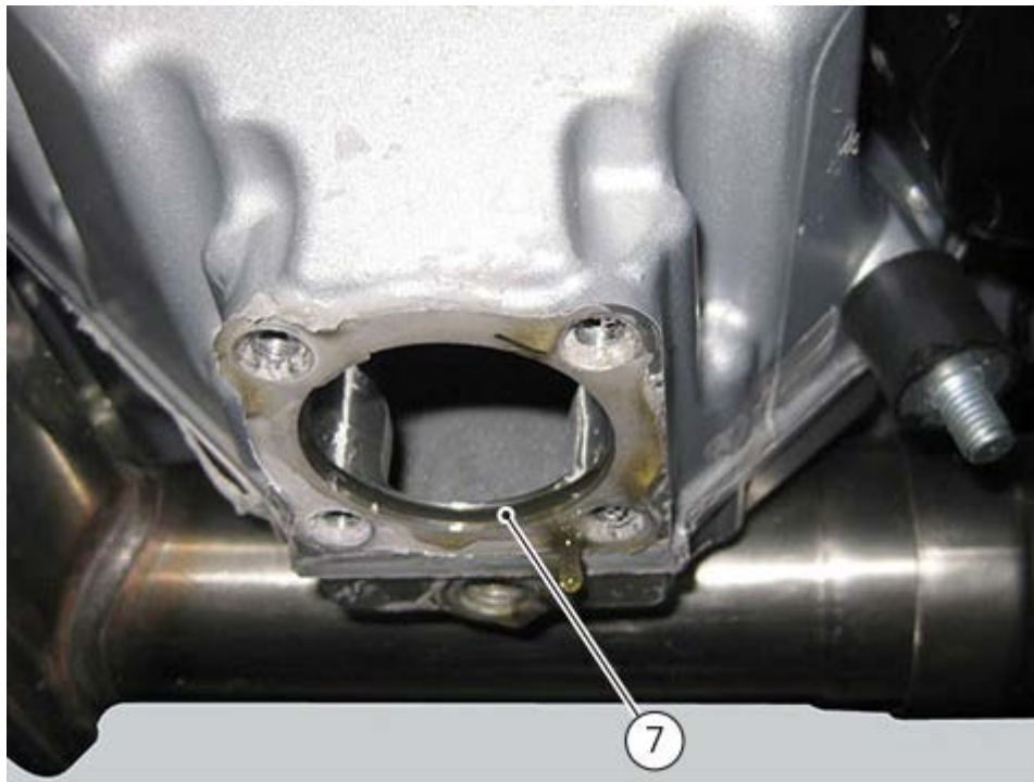
Position O-ring (7) on the crankcase and O-ring (6) on the mesh filter (5).
