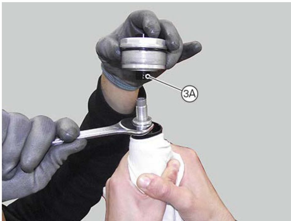
Tighten the upper plug (3A) on the damper rod while holding lock nut (2A) with a wrench.
