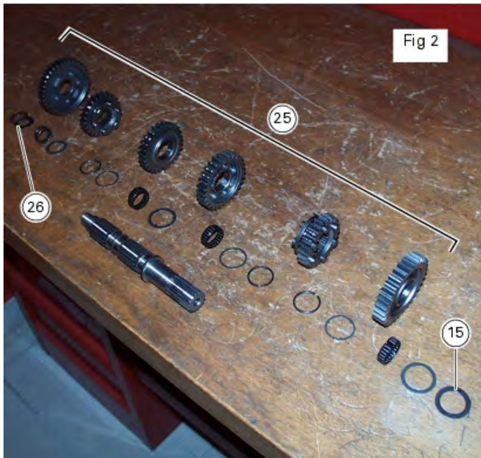
Fig. 2 shows all parts to be fitted onto the secondary shaft (25), after calculating correct thickness for shims (15) and (26) (Sect. N 9.2, Shimming the shafts ).
