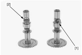
Apply molybdenum oil solution to the camshaft [1] lobes and journal surfaces.
