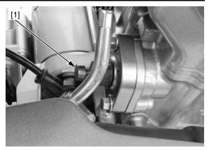
Apply engine oil to a new O-ring [1] and install it to the cam chain tensioner lifter.
