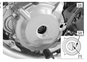
Make sure that the outside index lines ("IN" [1] and "EX" [2] marks) on the cam sprockets are flush with the cylinder head top surface and facing outward as shown.
