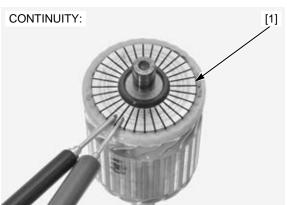
Check for continuity between each individual commutator bar [1] and the armature shaft [2]. There should be no continuity.
