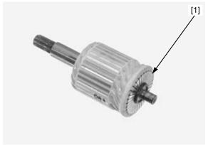
Check for continuity between pair of commutator bars
