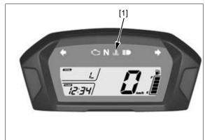
If the high coolant temperature indicator does not come ON at all or remains ON, inspect as follows.
