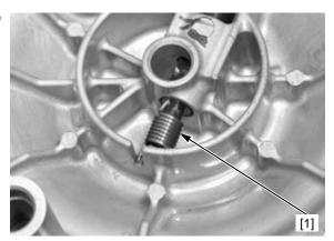
Remove the clutch lifter arm [1] from the right crankcase cover.
