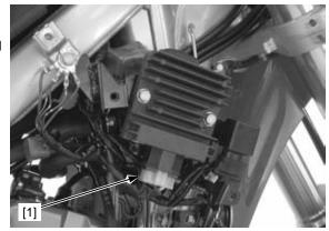
If the charging voltage reading (page 19-5) is out of the specification, check the following at the wire harness side connector [1]:
