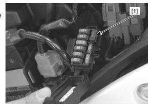
Check for continuity between the neutral diode terminals.
