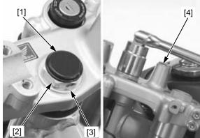
Loosen the steering stem adjusting nut [1] using the special tool.
