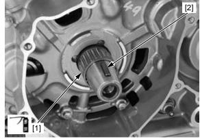
Install the flywheel while aligning the woodruff key on the crankshaft with flywheel keyway.
