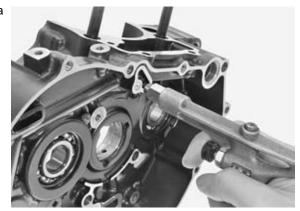
Clean the left and right crankcase mating surfaces thoroughly, being careful not to damage them and check for damage.
