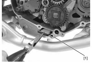
Install the oil strainer screen with the thin edge facing in and flange side facing up as shown.
