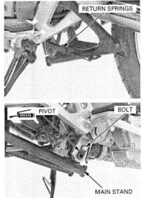
Remove the bolt and main stand pivot. Remove the main stand.
