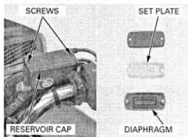
Fill the reservoir with DOT 4 brake fluid from a sealed container to the casting ledge.
