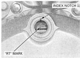
When checking the clearance, slide the feeler gauge from the center toward the outside.
