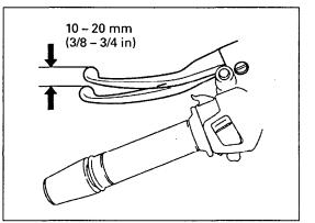
Minor adjustment is made with the upper adjuster at the clutch lever.
