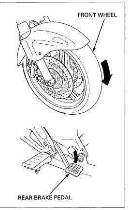
Firmly apply the brake lever or pedal, and check that no air has entered the system.
