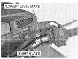
If the fluid level is near the "LOWER" level mark, remove the screws, reservoir cap, set plate and diaphragm.
