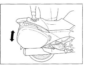
Support the motorcycle securely and raise the rear wheel off the ground.
