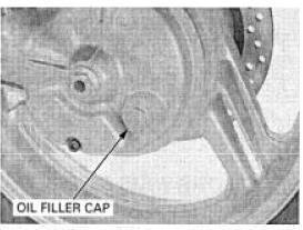
Check that the oil level is up to the lower edge of the oil filler hole.
