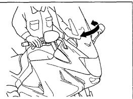
Check for steering stem bearings by grabbing the fork legs and attempting to move the front fork side to side.
