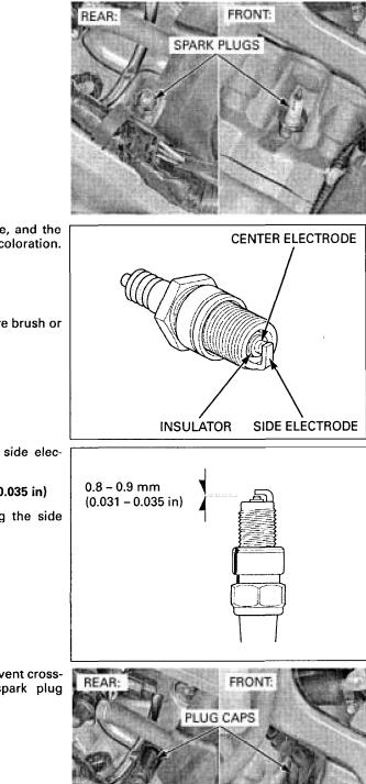
Check the insulator for cracks or damage, and the electrodes for wear, fouling or discoloration. Replace the plug if necessary.
