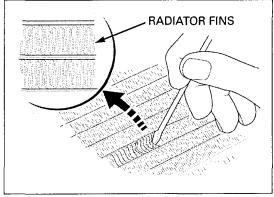
Straighten bent fins with a small, flat blade screwdriver and remove insects, mud or other obstructions with compressed air or low pressure water. Replace the radiator if the air flow is restricted over more than 20% of the radiating surface.
