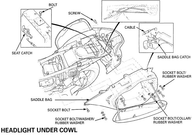
Remove the screws and headlight under cowl.
