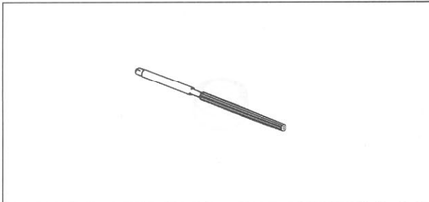
Valve Seat Cutter, 60^\circ - \phi 33 : 57001-1334
