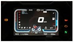
Rotation speed: The rotation speed of the engine. (r/min-Rotation/Minute----The rotation turning circles each minute of crankshaft)
