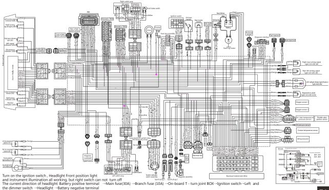
The current direction of position light and Instrument illumination: Battery positive terminal—Main fuse(30A) —Branch fuse (10A) —On-board T - turn joint BOX—Ignition switch—position light and Instrument illumination—Battery negative terminal
