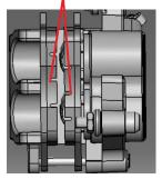
Limit abrasion position for rear brake pads:
