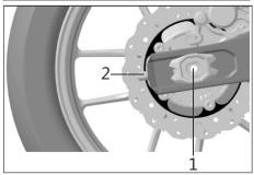
Fastening torque of adjusting nut: 14NM Fastening torque of rear wheel axle: 95NM
