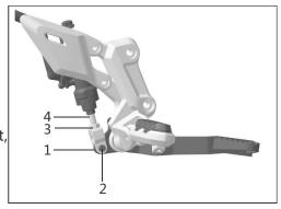
The free travel of rear brake pedal: 25-35mm The fastening torque for nut of adjusting stud: 18N.m
