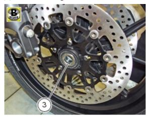
Install the complete wheel between the fork legs. Lubricate the shank and thread of the wheel axle (10).
