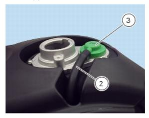
Release the breather valve (3) by turnig it anti-clockwiseand remove it from the fuel filler (8). Remove the fuel filler flange (8) by unscrewing the bolts (10) and recover the O-ring (9).
