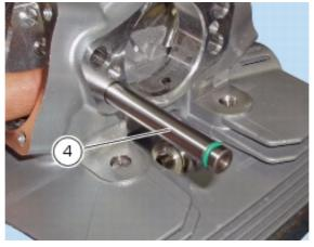
Detach the spring (9) and remove the tool 88713.2783.
