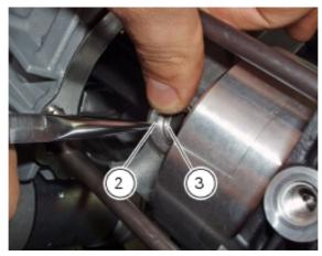
Working from the opposite side, drive out the gudgeon pin (3) sufficiently to release the connecting rod. Lift the cylinder/piston assembly clear of the engine crankcase studs.
