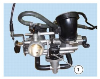
The stepper motor simultaneously controls two by-pass ports having an air flow capacity of around 6 kg/h.
