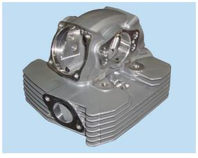
The cylinder barrel mating surface must be perfectly flat. If this is not the case, spread diamond dressing compound (6 to 12 micron thickness) on a reference surface and slide the cylinder head on the surface as shown in the figure until a flat finish is obtained.
