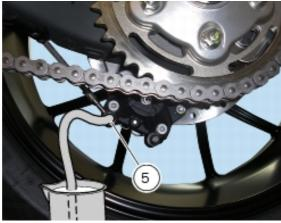
Unscrew the bleed valve by a 1/4 turn. Operate the brake lever (or pedal) until all the fluid has drained out. Repeat this operation for each brake caliper.
