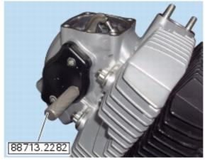
Remove the crankshaft locking tool 88713.2011 unscrewing first the pin and then the screw from the tool.
