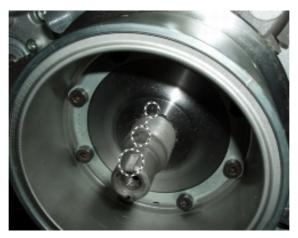
Lubricate the contact surfaces of Belleville washer (33) with engine oil. Fit the Belleville washer (33) on the end of the crankshaft.
