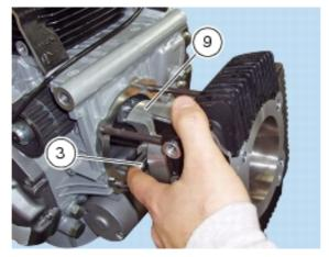
Stuff the crankcase opening with a cloth to prevent foreign objects from falling inside and then fit the circlip (2) using service tool **88713.2270**.
