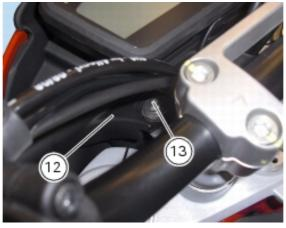
with the shorter thread should be facing the instrument panel. Fit the bush (18) to the centre rubber, screwing it on by hand.
