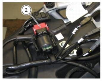
Insert the contactor in its seat on the fuel tank: the contactor must be inserted fully home, i.e. until the four retaining teeth of the support bracket protrude on the contactor side.
