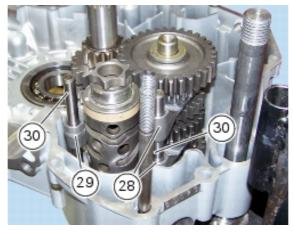
Remove gear selector forks (29) and (28).
