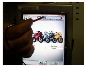
Press the icon "Select system" to display a list of the bike's systems that can be analysed. Select "Engine electronics" and press the "Confirm" icon (B).
