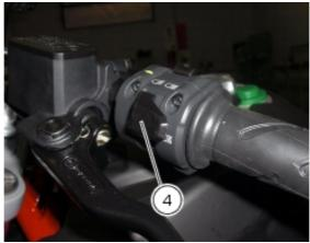
If the DDA function is active and the instrument panel is suddenly switched off (Key-Off), the function is automatically disabled.
