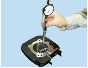
In the event of damage or excessive wear the barrel must be renewed as it has a silicon carbide coating (which provides the cylinder walls with excellent anti-friction and anti-wear properties) and therefore cannot be rebored. The cylinders are marked by a letter (punched into the specific surface on the cylinder side) showing the class to which they belong.
