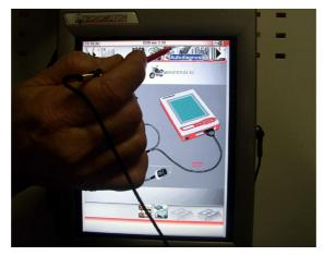
The DDS tester will interrogate the electronic control unit and display the parameters analysed with their relative values.
