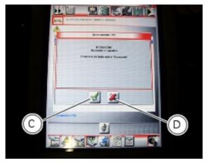
Once the reset has been performed, the ECU will be associated with the motorcycle's throttle body. Replacement of the throttle body, the throttle position sensor or the ECU must always be immediately followed by a new reset procedure.
