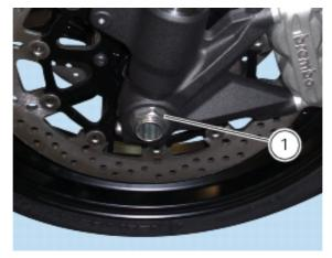
Loosen the axle clamp bolts (11) on the ends of the fork legs.
