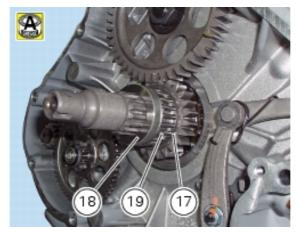
Install the flywheel-rotor-driven gear assembly on the crankshaft, taking care not to alter the position of the inner race (18) relative to the washer (17).
