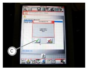
If any problems were encountered during the operation, the tester will display the relative error messages: each message must be confirmed, (by pressing the "Confirm" icon (C)), or rejected (by pressing the "Exit" icon (D)).
