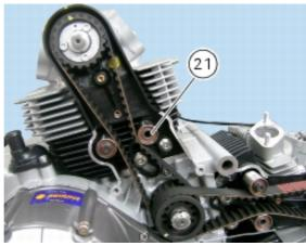
Check the timing belt tension and adjust if necessary as described in the paragraph "Measuring timing belt tension" (Sect. D 5).
