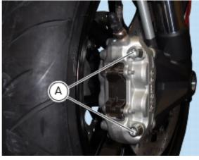
Check that the brake discs turn freely inside the calipers.
