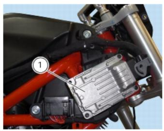
It controls both the injectors and the coils, thus controlling fuel injection and ignition in accordance with the engine operating conditions detected by the following sensors:
