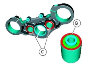
Locate the lower clamps (8) on the top yoke. Fit the bolts (2) in the clamps (8), screw on the nuts (9) complete with washers (7) and (10). Tighten the bolts (2) to the specified torque (Sect. C 3, <a href="Frame torque settings">Frame torque settings</a>) while counterholding the nuts (9). Position the handlebar (4) in its seat on the lower clamps (8).
