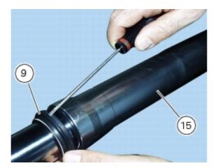
Remove the circlip (10).
