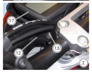
Withdraw the headlight support (12) towards the front and disconnect the headlight wiring (Sect. P 1, Routing of wiring on frame).
