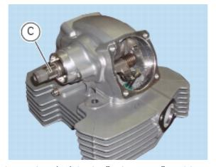
Using two screwdrivers, hold the closing rocker (18) in the "valve open" position.
