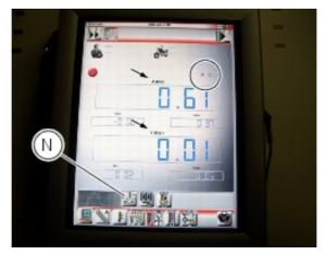
The measured value is indicated alongside the letter (A) or (C) identifying the cable used for the measurement: i.e. if you used connector (A) of the cable (3), the value measured will displayed next to the letter (A) on the screen. The maximum pressure must be **3** bar (nominal).
