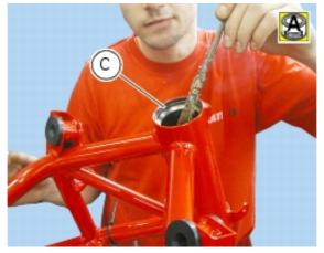
To fit the outer races (C) of the bearings (5) and (6) to the steering head, use the service tool no. 88713.1062 and proceed as follows:
