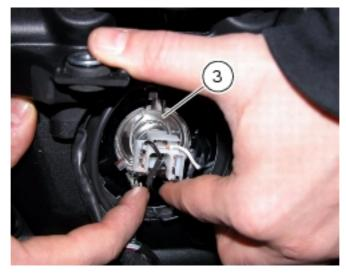
The bulb (4) is of the bayonet-type: press and twist anti-clockwise to remove. Push in the new bulb and turn it clockwise until it clicks into place.
