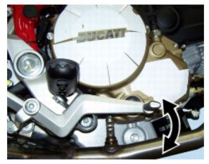
Attach a length of transparent plastic tubing to the bleed valve (2) and insert the other end of the tubing in a container placed on the floor.
