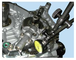
Position the dial gauge stylus on one tooth of oil pump gear and set the gauge to zero in this position. Move the gear slightly to measure the backlash; take four readings in diametrically opposed positions of the gear. The backlash should be **0.10** mm.
