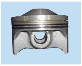
Clean the piston crown and piston ring grooves, removing any carbon deposits. Inspect the piston and check its dimensions carefully: there must be no signs of scuffing, scoring, cracks, or other damage.
