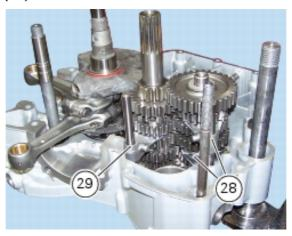
Remove the gearbox input (2) and output (25) shafts complete with gears, taking care to recover the spacers on the ends of the shafts.
