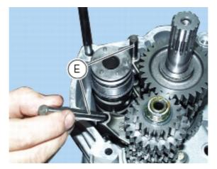
Fit the shimmed crankshaft into the clutch-side crankcase half, positioning the connecting rods (E) in correspondence with the relative cylinder barrel seats.
