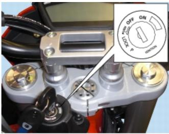
Check the neutral indicator light N (3), and the red oil pressure warning light (4) on the instrument panel are both illuminated (Sect. P 7, <u>Instrument panel system</u>) and that the engine stop switch (1) is in the position (RUN), then press the starter button (2). Allow the engine to start on its own, without turning the throttle twistgrip.
