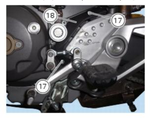
Renewal of the oil seal on the gearbox output shaft
