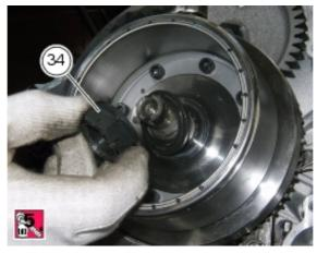
Restrain the rotation of the flywheel with the holding tool 88713.2036.
