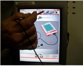
The DDS tester will interrogate the electronic control unit and display the parameters analysed with their relative values.
