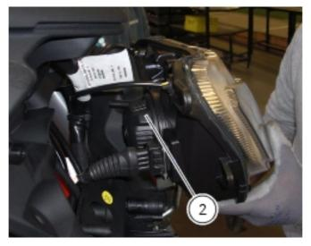
Reposition the headlight support on the motorcycle and refit the bolts (1) to the frame.
