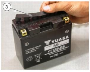
For 3-12 Ah batteries, leave to stand for at least 30 mins. For batteries of over 12 Ah, leave to stand for at least 1 hour.
