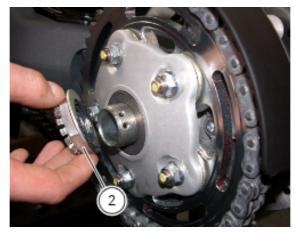
Fully unscrew the nut (2) and remove the washer (3) and the flange (5) complete with the rear sprocket.
