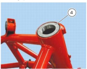
Grease adjusting ring nut (3) and tighten it by hand up against the oil seal (4). Fit service bush no. **88713.1058** to the steering stem nut (3) and fit the torque wrench to the bush. Tighten the steering stem nut (3) to the specified torque (Sect. C 3, Frame torque settings).
