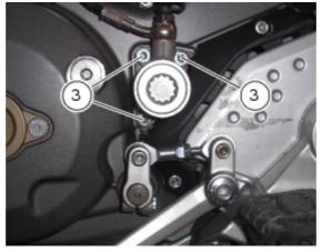
Remove the clutch slave cylinder (4) taking care not to damage the internal O-ring (5). Push in the piston to force out all the fluid from inside the slave cylinder.
