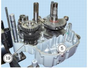
Apply a uniform and continuous bead of DUCATI liquid gasket to the mating surfaces of the crankcase halves, going around all the holes as shown in the figure.
