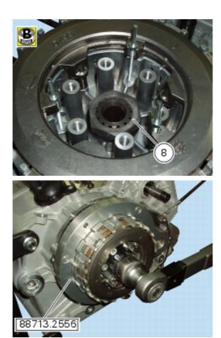
Install the pressure plate (5) in the clutch asembly (B) aligning the three tools **88713.2591** with the three indents (N) in the pressure plate.
