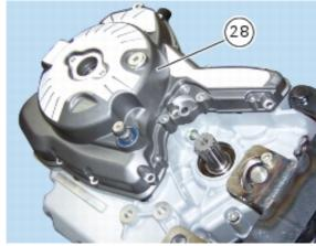
Insert the retaining bolts in their holes following the indications given in the table.
