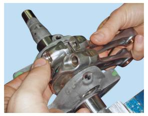
Use the recommended grease to lubricate the threads and underside of the heads of the new bolts (8) and the threaded hole in the connecting rod, packing in grease from both sides of the hole.
