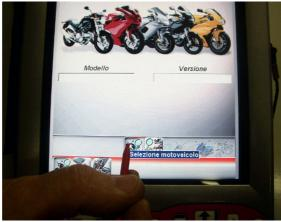
Press the icon "Select system" to display a list of the bike's systems that can be analysed.
