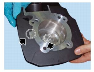
If the pistons have been separated from their cylinders, before reassembling these components, position the piston ring gaps at 120° from one another (the markings must always face the piston crown). Use a universal tool to carefully insert the piston into the cylinder (first lubricate the inside of the cylinder with engine oil). Position the cylinder with the smallest valve pockets facing the exhaust port.
