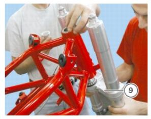
Grease the ball race (B) and fit it to outer race (C) of the top bearing.
