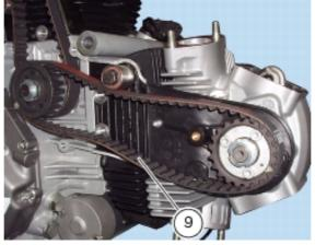
Locate the tensioner pulleys (21) on the vertical and horizontal cylinders. Screw in, but do not tighten at this point, the screws (27) and (20), so that the tensioner pulleys can rotate.
