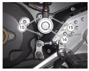
Locate the hose (6) on the slave cylinder (14), ensuring that the hose end fitting is correctly positioned relative to the slave cylinder (14).
