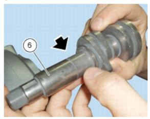
Apply graphite oil to the seats of the camshaft so that it is lubricated also during the initial revs of the engine. Insert the camshaft (16) from the left-hand side of the cylinder head.
