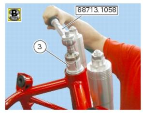
Fit the top yoke (2) on the steering stem nut (3), aligning the fork leg bores with the corresponding bores on the bottom yoke. Relocate the fork legs as described in Section G 2, <u>Refitting the front forks</u>.
