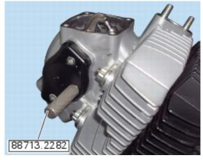
Turn the pulleys by hand until the end of the tool engages the slot in the camshaft.
