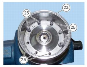
Insert two of the bolts (25) just removed from flywheel rotor-side in their holes in order to remove the flange (13) and the starter clutch (21) from the flywheel (16).
