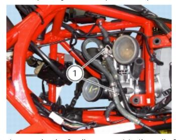
The control unit controls injector opening by feeding current to the coil of an electromagnet which
