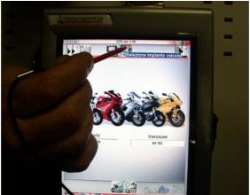
A list of the motorcycle's systems that can be analysed will appear on the display. Select "Engine electronics". Press the "Confirm" icon (C).
