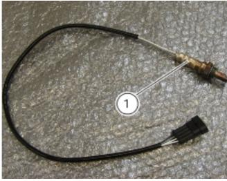
The outer surface of the sensor element in zirconium dioxide is in direct contact with the exhaust gas, while the inner surface is in contact with the atmosphere. Both surfaces are coated with a thin layer of platinum. Oxygen in ionic form travels through the ceramic layer and charges the platinum layer electrostatically so that the platinum acts as an electrode: the electrical signal generated is carried on the sensor output cable.
