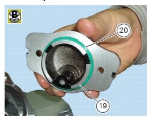
Secure the end cap (20) with the bolts (21). Tighten the bolts (21) to the specified torque (Sect. C 3, <u>Engine torque settings</u>).
