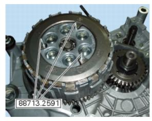
Unscrew the retaining screws (1) and remove the collars (2) and the clutch springs (4).
