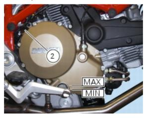
Check for oil leaks. Check that the oil pressure light on the instrument panel switches off a few seconds after the engine starts. If not, switch off the engine and trace the fault.
