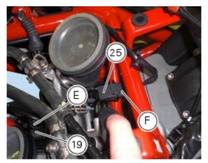
Remove the throttle body assembly (11) from the motorcycle.
