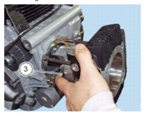
If work is to be carried out on the piston, carefully withdraw it from the cylinder.
