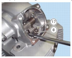
Position the two half rings (7) on the valve stem. Remove the screwdriver and position the closing rocker arm (18) in the rest position.
