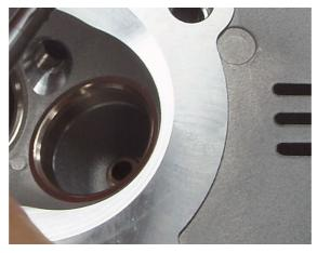
Allow to cool and then lap the valve seats, smooth the connections between the ducts and the new seats and grind the valves.
