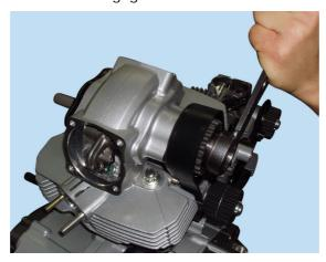
Fit the horizontal (9) and vertical (23) timing belts using your hands only and without altering the alignment of the pulleys.
