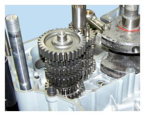
Install the selector forks of the  $1^{St}$ - $4^{th}$  and  $2^{nd}$ - $3^{rd}$  gears (B) in their respective grooves in the output shaft driven gears.
