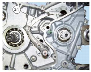
Fit the bolts (18) and (20) with the spacer (19). Temporarily fit the gearchange lever (or a service lever) and the front sprocket, and put the gearbox in neutral.
