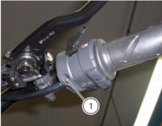
Checking the right-hand handlebar switch
