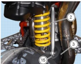
On removing the lower bolt (15), the lower ball-joint end fitting (6) of the tie-rod (2) is also released from the swingarm. Recover the threaded bush (16) and the bushes (4) located either side of the lower ball joint of the tie-rod.
