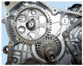
Check that the Woodruff key (1) on the timing gear driveshaft and the Woodruff key (5) on the crankshaft are both present.
