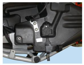
Refit the bracket (G), apply the recommended threadlocker and tighten the bolts (H) to the specified torque (Sect. C 3, Frame torque settings).
