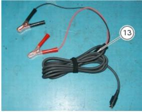
connect the power and diagnostic cable (2) to the diagnostic connection socket (N) on the tester; then connect the -battery socket adapter (8) to the connection socket (R) on the power and diagnostics cable (2) and to the motorcycle battery;
