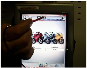
Press the icon "Select system" to display a list of the bike's systems that can be analysed. Select "Engine electronics" and press the "Confirm" icon (B). Next, press the "Self-diagnosis" icon to access the corresponding function.
