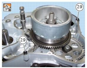
Spread a continuous uniform bead of DUCATI liquid gasket on the mating surface of the cover (28), ensuring continuity around the holes for the retaining bolts and locating bushes.
