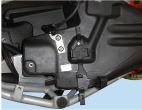
Remove the fuel tank (1) from the motorcycle.
