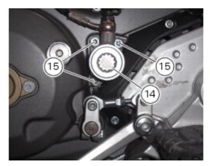
Remove the dust cap (12) and the bleed valve (11) and unscrew the banjo bolt (10), taking care to recover the sealing washers (8): the unit (14) is now disconnected from hose (6). Push in the piston to force out all the fluid from inside the cap.
