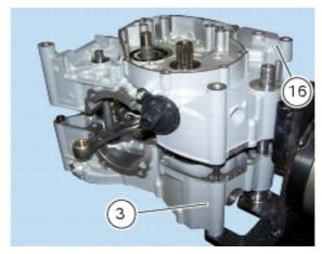
Prepare the crankcase bolts, and insert them in the alternator-side crankcase half (3); note that the bolts are of different lengths.
