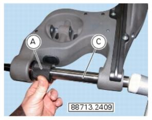
Drive the bearing (2) fully into the swingarm.
