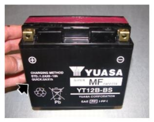
Charge the battery if the open circuit voltage is lower than **12.8** V. Leaving the battery discharged for more than one month could damage it. Check the battery charge with a voltmeter.
