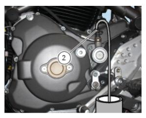
Draining the clutch hydraulic circuit
