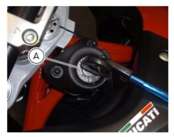
turn the key to OFF and connect a multimeter to contacts (1) and (4) to check electrical continuity - (Sect. P 9, <u>Diagnostic instruments</u> concerning operation of the multimeter). The resistance reading should be near zero and, if present, the audible continuity signal should be emitted;
