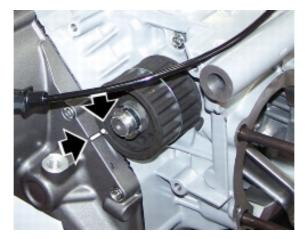
Set the degree wheel of service tool no. **88713.0123** to zero the horizontal cylinder is at top dead centre of the expansion stroke, and therefore we can proceed to check the valve clearances on this cylinder.
