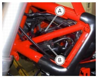
Unscrew the nuts (1) securing the ignition switch cover (2) and remove it along with the immobilizer antenna.
