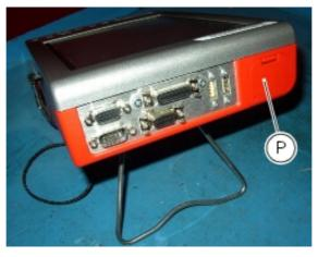
When using the tester, take care never to allow the power supply to fall below the minimum voltage: this situation could occur during engine starting and idling on motorcycles in which the battery is not in perfect working order. If the tester detects a power supply voltage of less than **9** Volts, the current procedures will be aborted; when the voltage returns to within the acceptable tolerance limits the procedure must initiated again from the beginning.
