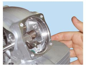
Install the valve (17) and valves (16), first lubricating them with engine oil.
