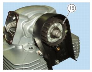
Fit the tool no. **88713.3152** onto the pulleys to prevent rotation. Apply a smear of grease to the thread and underside of the nut (13), and fit the washer (14) and the nut.
