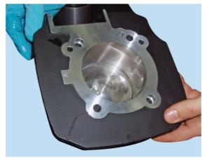
To remove the vertical cylinder-piston assembly, proceed as described above for the horizontal cylinder. Remove the cylinder-crankcase gaskets (6) from the cylinder barrel.
