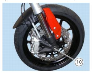
Remove the wheel and recover the spacers (3) and (9).
