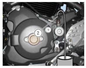
Open the bleed valve (2) a 1/4 turn and operate the clutch lever several times until the fluid starts to emerge from the bleed valve (2).
