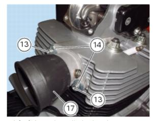
If necessary, remove the studs (12) and (13) from the cylinder heads.
