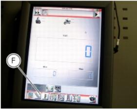
The socket to which the cable (Measurement Module) (3) is to be connected is indicated on the screen with a capital letter: A, B or C.
