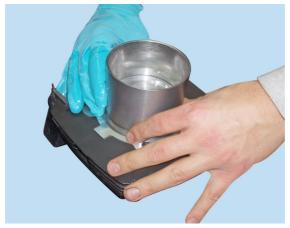
Remove any deposits and degrease the contact surfaces of the crankcase and the cylinders. Check that the dowel (1) is installed on the crankcase.
