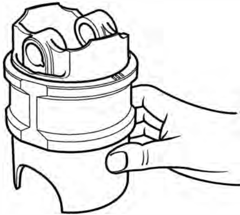
Aligning Piston Rings using the Piston
